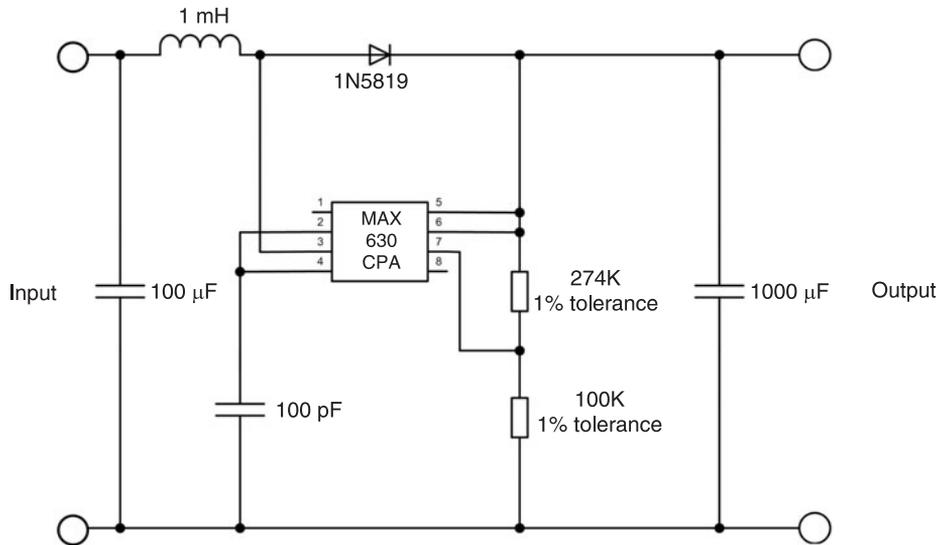
Figure 13-45 DC-DC converter board schematic.
