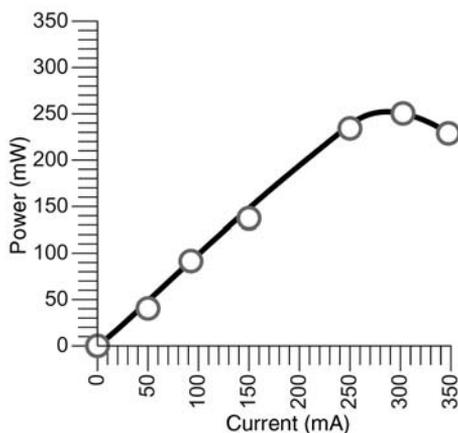
Figure 6-23 Example power curve graph.
