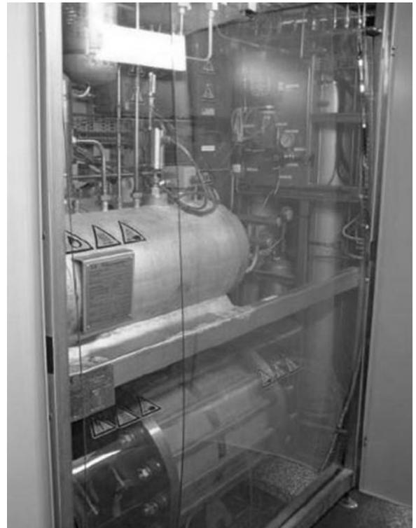
Figure 3-13 The HARI electrolyzer. Image courtesy Dr Rupert Gammon
