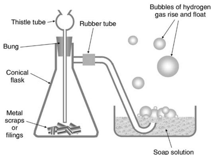
Figure 14-5 *Making hydrogen bubbles.*
