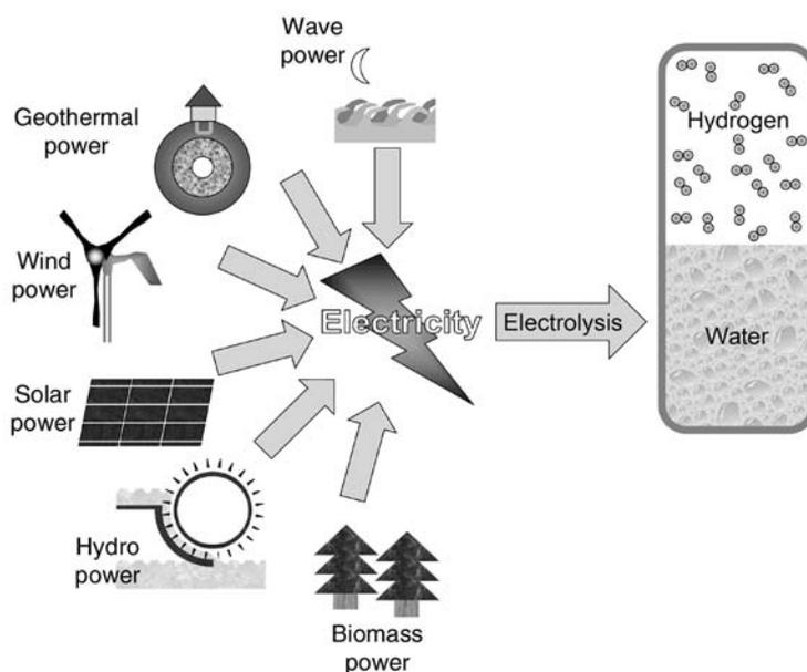
Figure 2-5 *Hydrogen produced from clean, renewable energy.*
