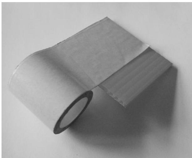
**Figure 13-47** *Cover the plastic platform with double-sided tape.*
