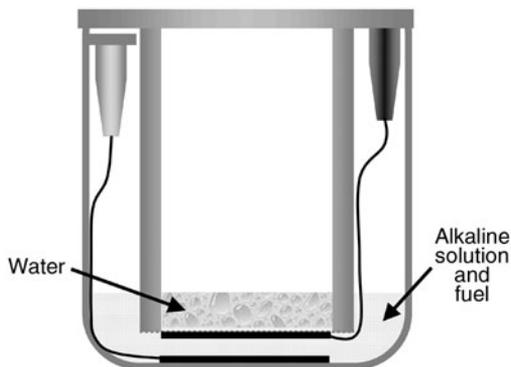
Figure 6-27 *The water blocks oxygen.*
