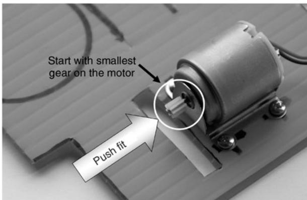
Figure 13-22 The smallest gear should be a push-fit on the motor shaft.
