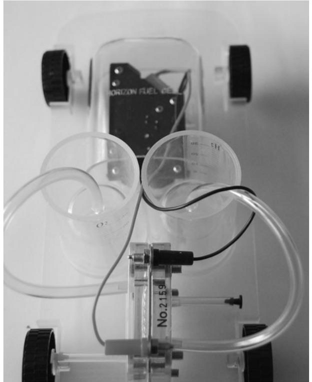
Figure 13-37 Fuel cell connected to the motor.
