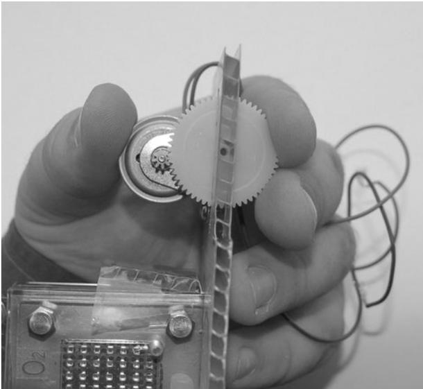
Figure 13-25 Align the axle hole with the corrugated plastic holes.
