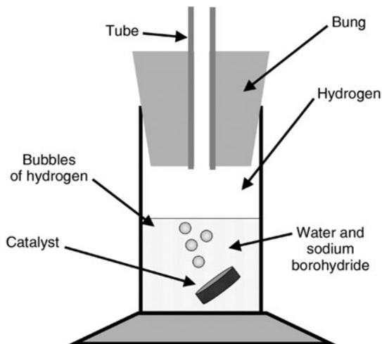
Figure 4-18 Diagram showing the H-Gen producing hydrogen gas.
