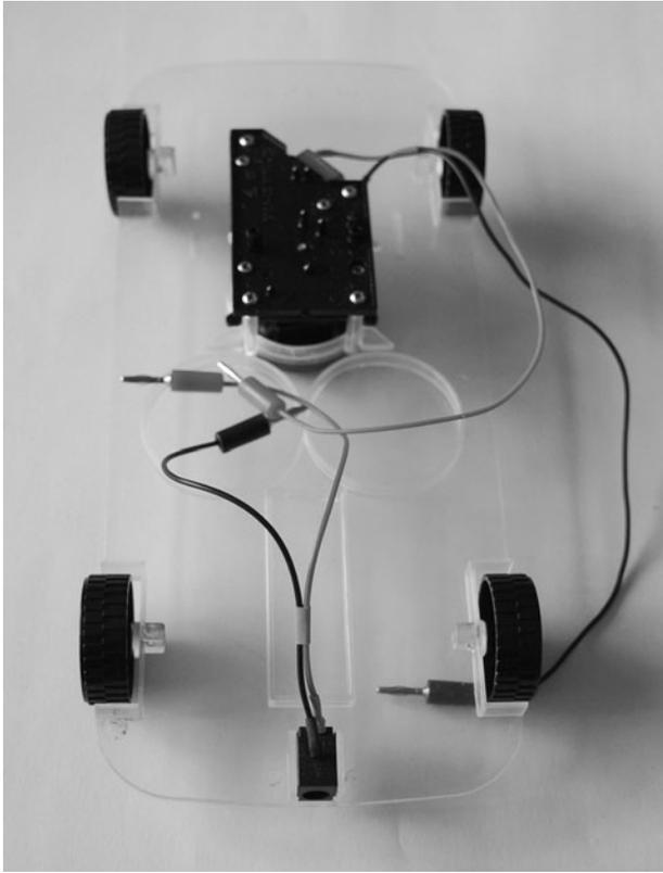
Figure 13-32 *Wheels installed.*
