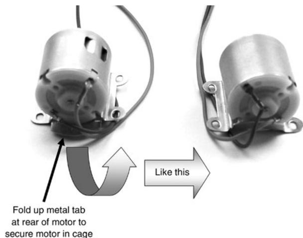
Figure 13-14 *Fold the tab to secure the motor.*
