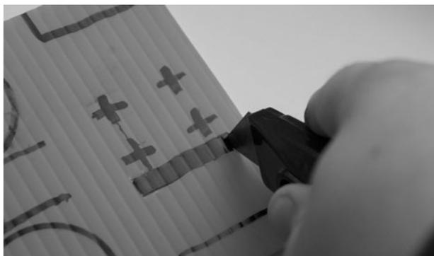
Figure 13-18 Use a sharp craft knife to cut through both layers of the plastic.
