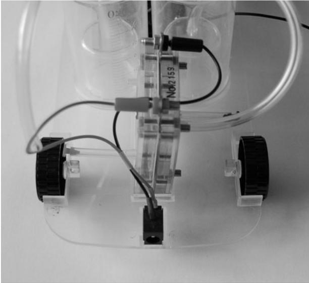
Figure 13-36 Fuel cell connected to the battery slot.
