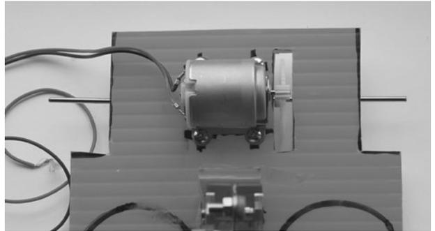
Figure 13-27 Axle and large gear wheel installed.
