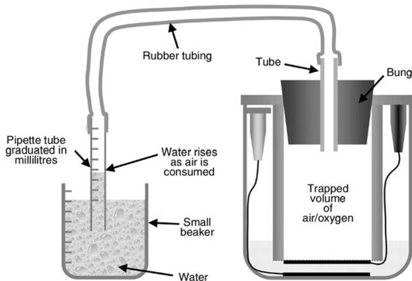
Figure 6-29 The oxygen consumption measurement apparatus.
