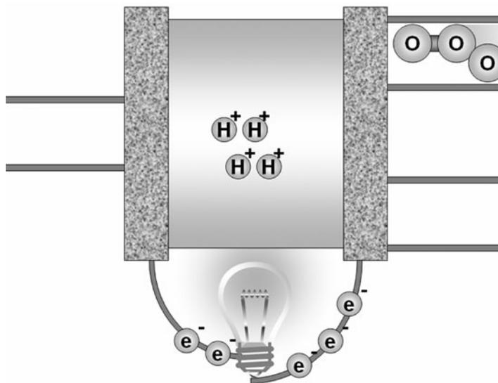
Figure 7-4 *Oxygen enters the fuel cell.*
