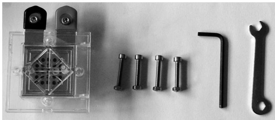
**Figure 7-16** *The fuel cell with fixings removed.*
