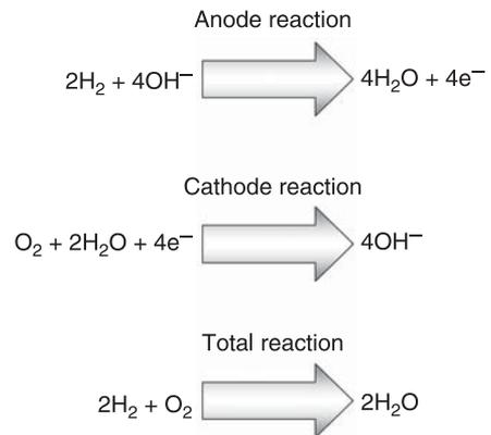
Figure 6-2 The chemistry of alkaline fuel cells.
