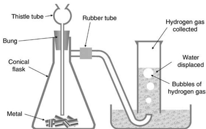
Figure 3-3 Producing hydrogen from acid and metal.
