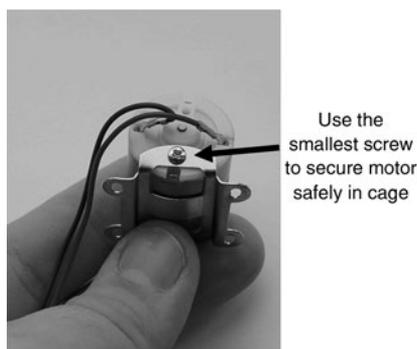
Figure 13-15 *A screw secures the motor in the cage.*
