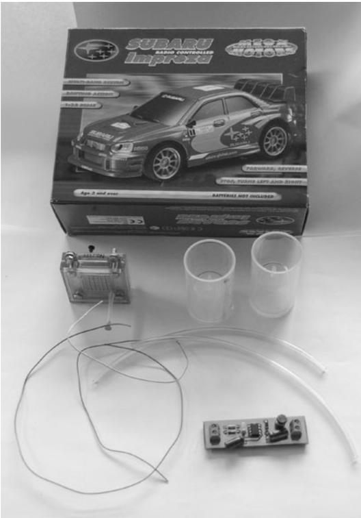
Figure 13-40 Components for RC fuel cell car.
