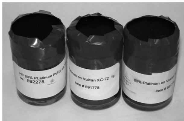
Figure 11-13 Jars of anode and cathode pastes.
