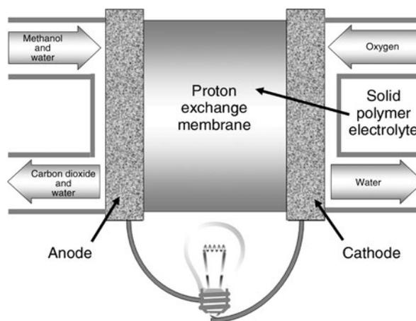
Figure 8-2 Direct methanol fuel cell diagram.
