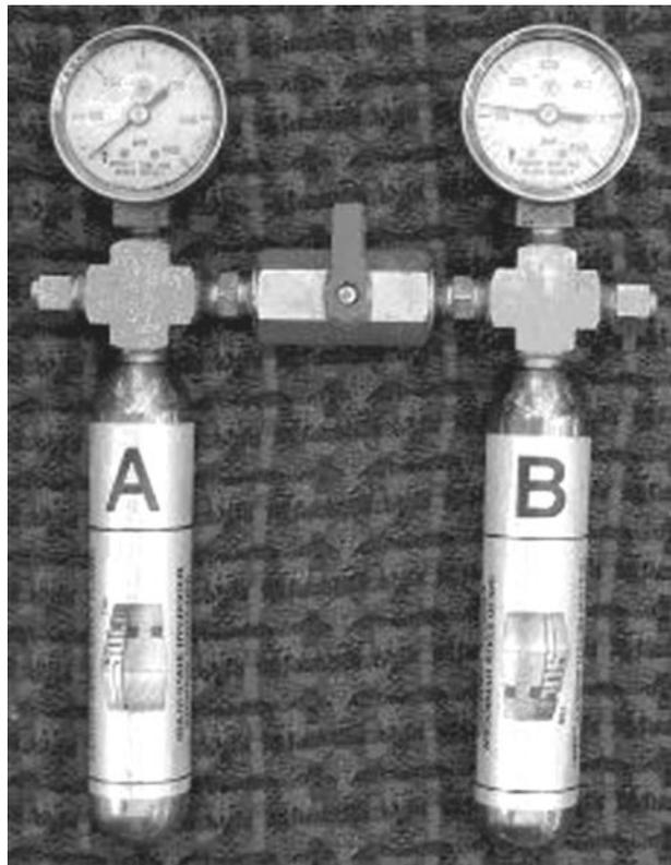
Figure 4-20 Apparatus for experimenting with metal hydrides.
