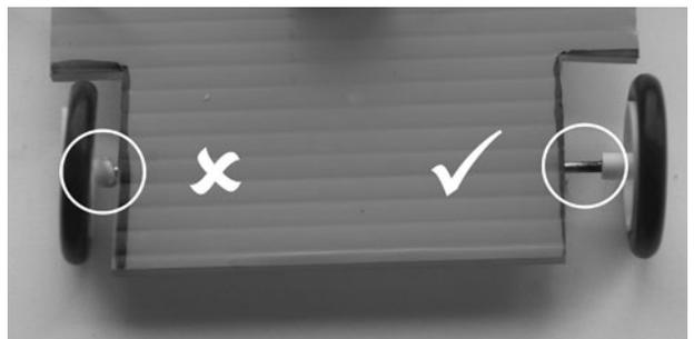
Figure 13-28 Heat the axle not the wheel.
