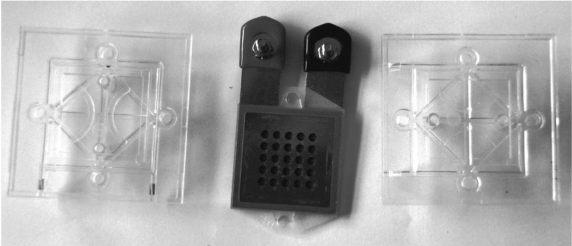
Figure 7-18 The end plates and electrode assembly.
