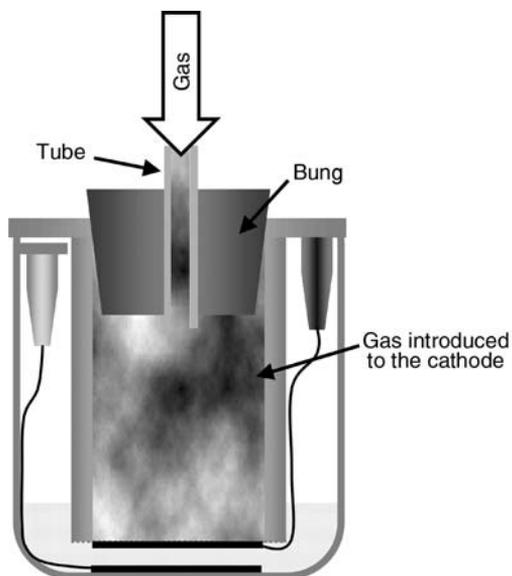
Figure 6-28 A bung and pipe allow you to introduce different gases to the AFC's anode.
