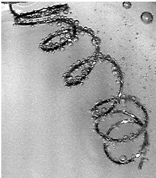
Figure 5-9b Close-up of the hydrogen electrode.
