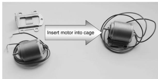
Figure 13-13 Insert the motor in the cage.
