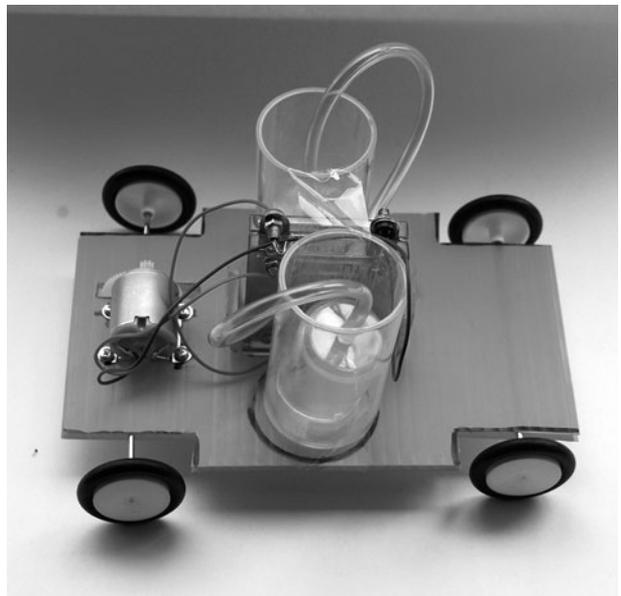
Figure 13-30 *Simple fuel cell car complete (side view).*
