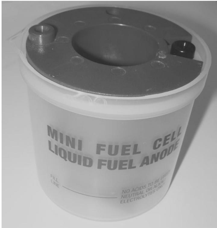
Figure 6-6 The assembled mini alkaline fuel cell.
