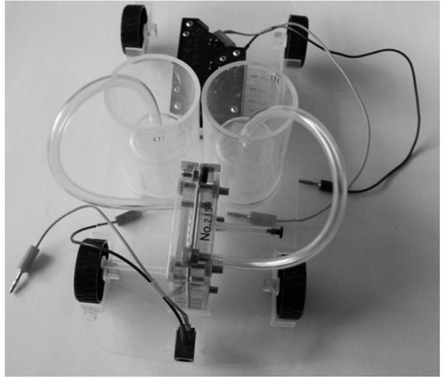
Figure 13-34 *Fuel cells and tanks installed.*
