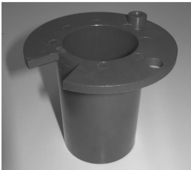
Figure 6-9 The mini alkaline fuel cell cathode assembly.
