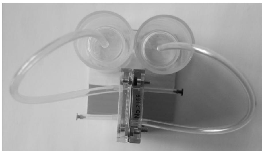
**Figure 13-48** *The hydrogen fuel cell power unit.*
