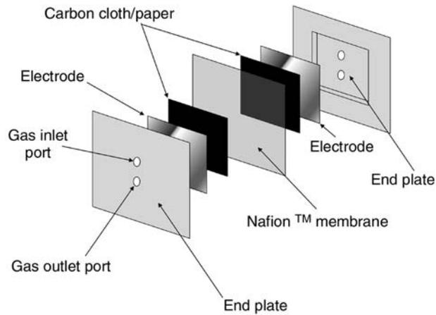
Figure 7-23 Diagram showing the components of your dismantlable fuel cell.
