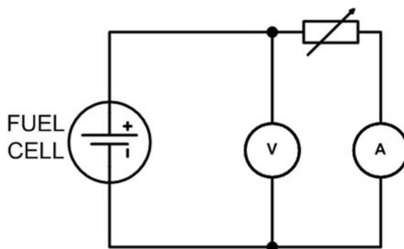
Figure 6-19 Schematic diagram for the alkaline fuel cell measurement setup.
