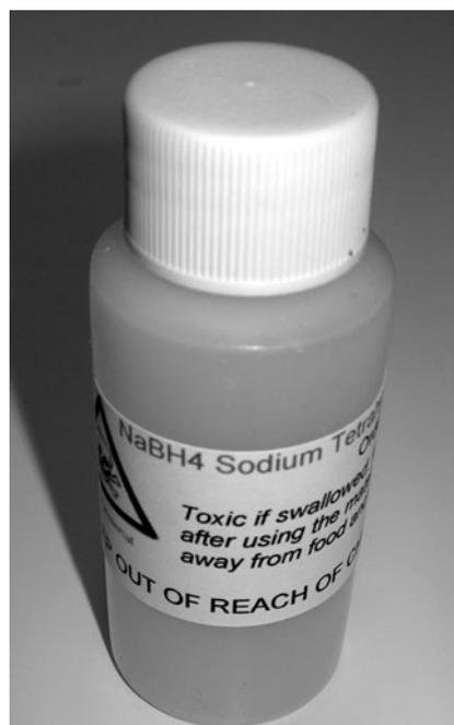
Figure 6-12 Sodium borohydride, the source of hydrogen for our AFC.
