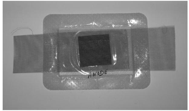
Figure 8-19 Laying the final layer of wire mesh on top of the MEA.
