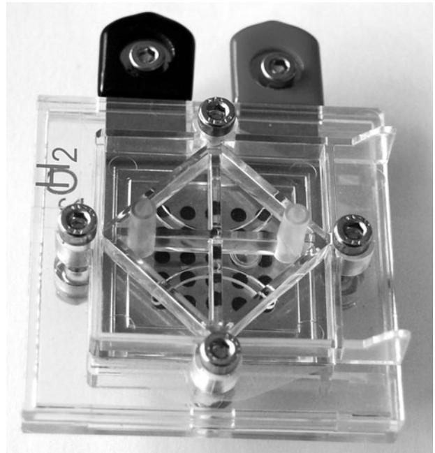
Figure 7-14 *The complete dismantlable fuel cell.*
