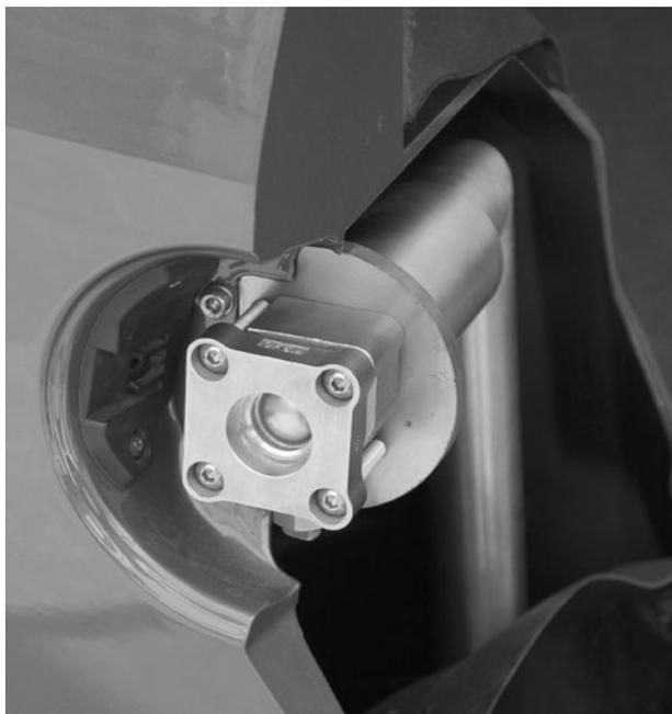
Figure 13-6 *A hydrogen coupling on a car.*
