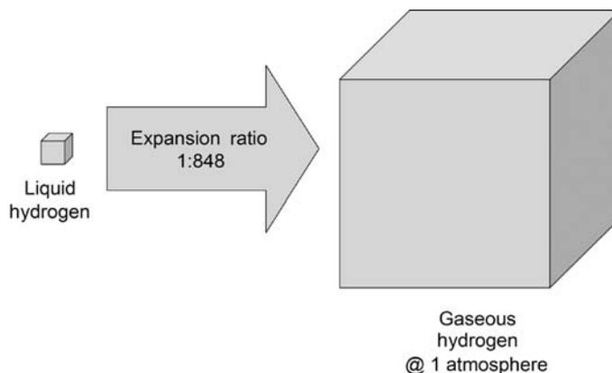
Figure 2-3 The expansion ratio of hydrogen.
