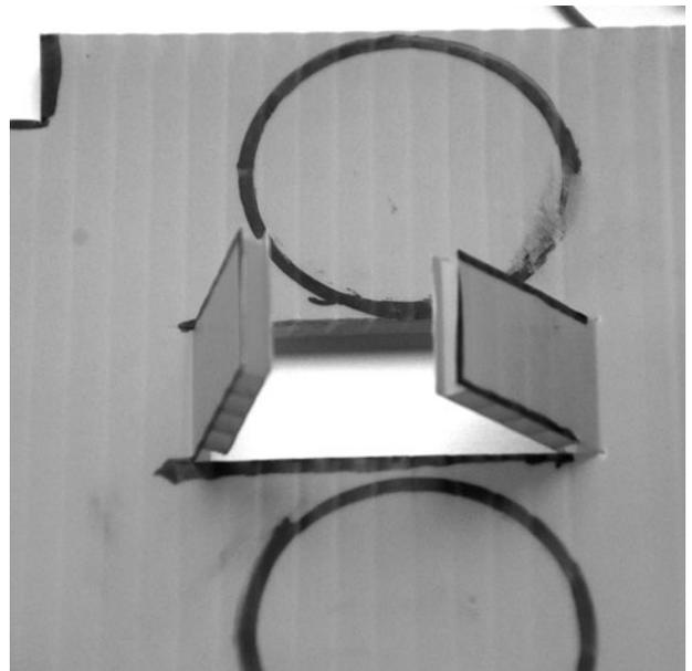
Figure 13-23 Fold the fuel cell support flaps up.
