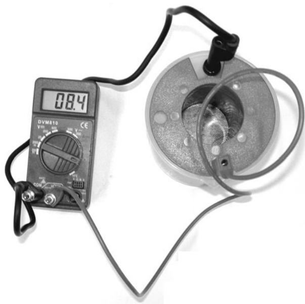
Figure 6-16 The alkaline fuel cell connected to the voltmeter.
