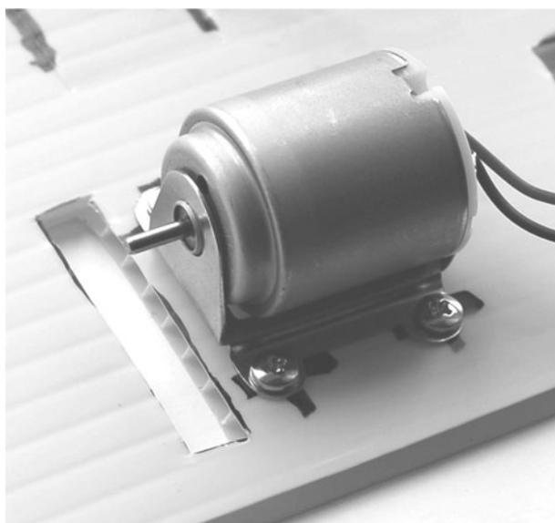
Figure 13-20 Motor mounted with shaft above gear-slot.
