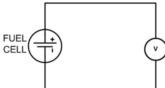
Figure 6-17 Schematic for connecting the AFC to the voltmeter.
