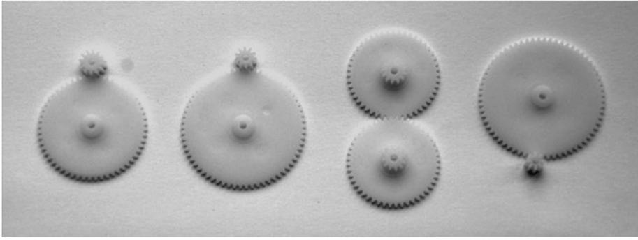
Figure 13-21 Combine the gears to make different ratios.
