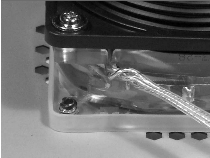
FIGURE 3-8: Fan noise reduction gasket assembly
