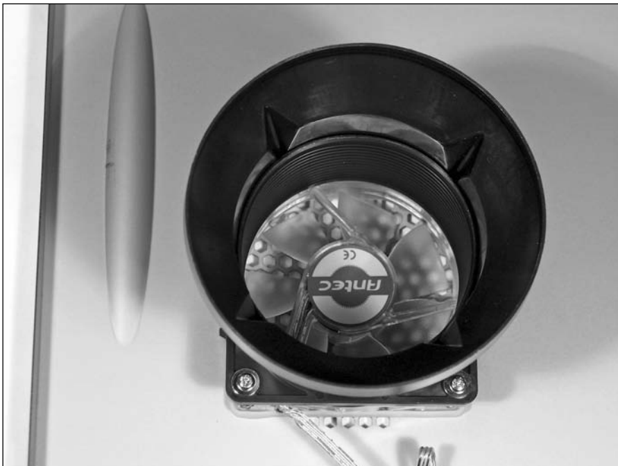
FIGURE 3-7: CPU cooling air duct with fan
