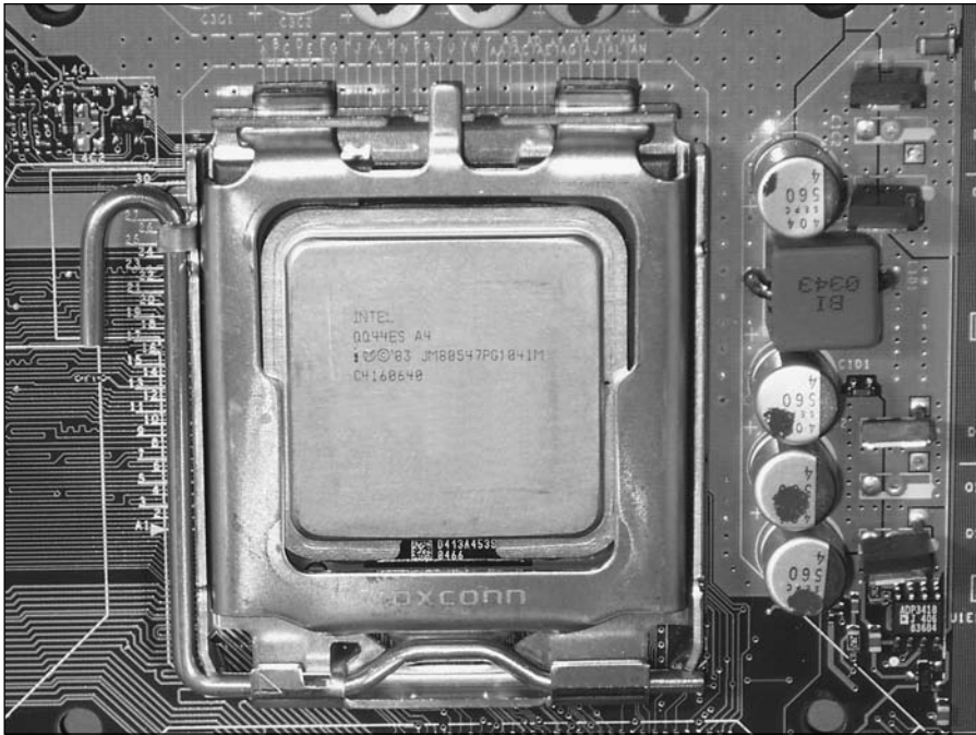
FIGURE 3-12: Pentium 4 processor installed in LGA775 socket
