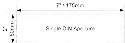
Figure 5-16 Dimensions for single-height DIN aperture
